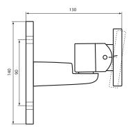
Dimensions in mm of included mounting bracket (with marked angle)
