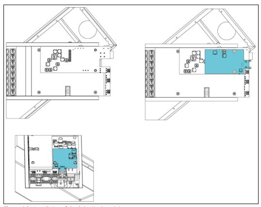
Figure 4.6 Installation of the CobraNet® module
