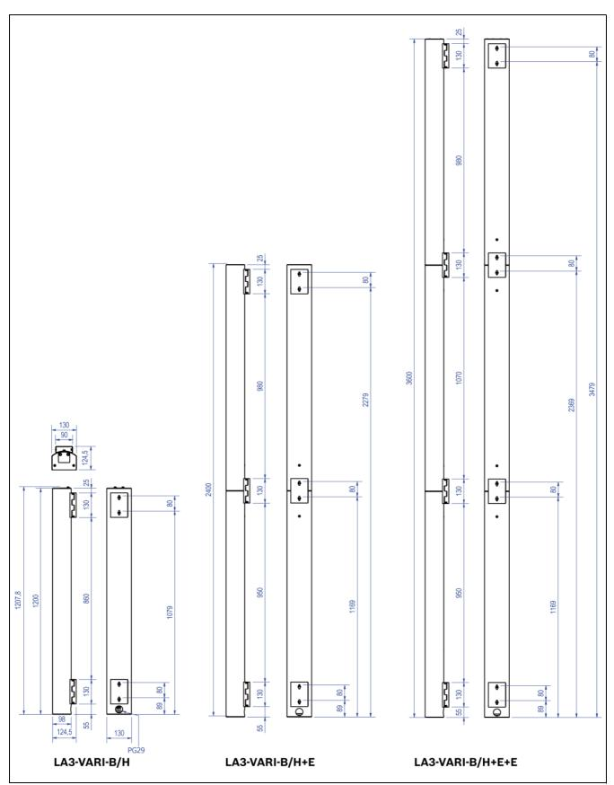
Figure 4.8 Mechanical dimensions in mm
