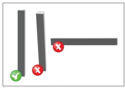
Figure 4.1 Upright loudspeaker mounting
