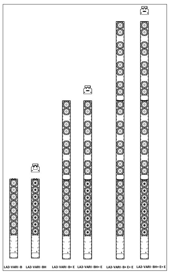
Figure 3.1 VARI overview (grilles removed for identification)
