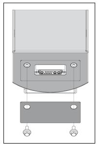
Figure 4.2 Removing D-shell connector coverplate
