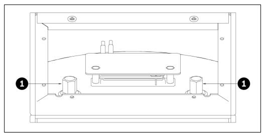
Figure 4.4 Access to fixing screws
