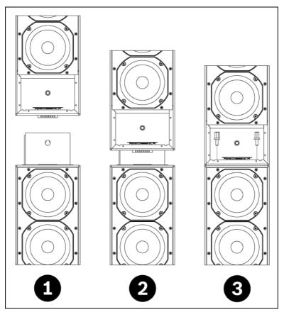
Figure 4.5 Mate extension unit to base unit
