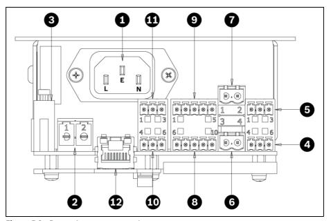
Figure 5.2 Base unit connector overview
