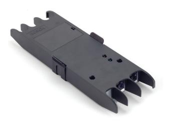
The network splitter is used in a network to provide two branches from the main cable run. It can use an external DC power supply, or it can use the power supply from the network controller. The unit automatically switches to the local power supply unit when it is connected to it, reducing the power drain on the main network. The network splitter can also function as a repeater, effectively extending the length of the main network another 50 meters.
