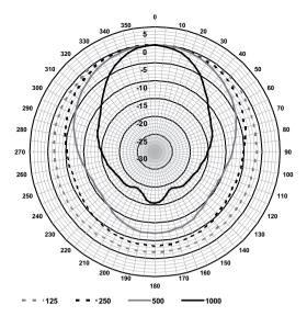
Horizontal polar diagram (pink noise octave, normalized at  $0^{\circ}$  axis)
