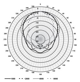
Vertical polar diagram (pink noise octave, normalized at  $0^{\circ}$  axis)
