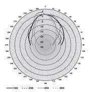
Vertical polar diagrams of LB3-PC350 (pink noise octave, normalized at  $0^{\circ}$  axis)
